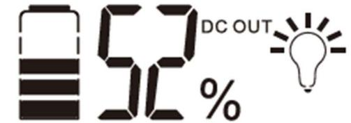
Figure 6. Digital Display when DC output is ON
