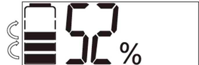
The display will show a **"charging motion"** when charging via solar panel(s) or AC power. The state of charge is shown by percentage, and by the battery icon. Each bar in the battery icon represents about 20% of charge. Once the battery is fully charged, the "charging motion" will stop, and the state of charge will remain at 100%.
