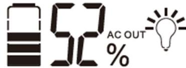
Figure 4. Digital Display when AC output is ON
